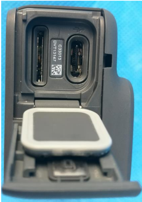
USB port and SD card port, SPTM1(Version S)
