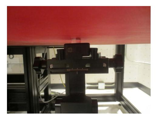
**1.2** Tablet Bottom Side with 10mm Spacer to the Flat Phantom Setup Photo
