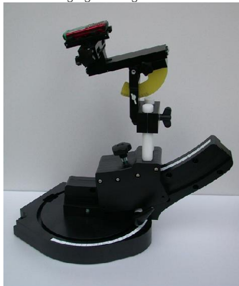
Device holder supplied by SPEAG
