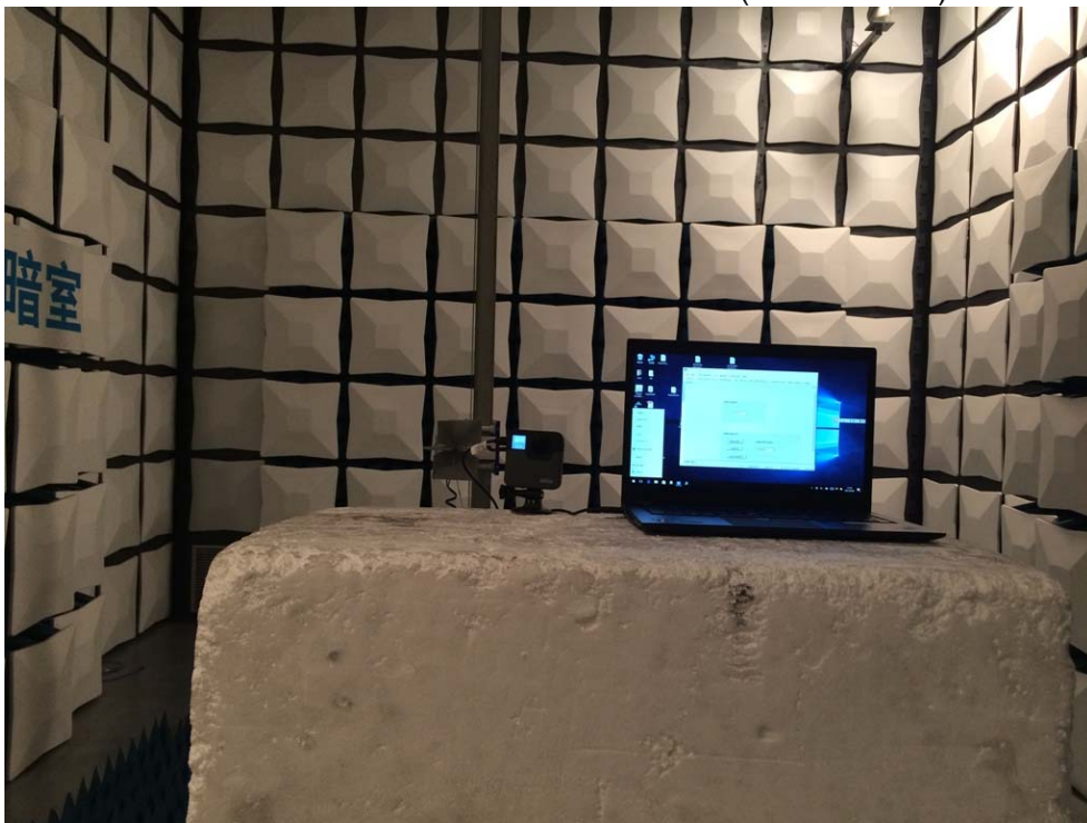
RADIATED RF MEASUREMENT SETUP (Above 1 GHz)
