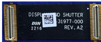
340-31973-000 ASSY, FPC, DISPLAY AND SHUTTER, CPPM1
