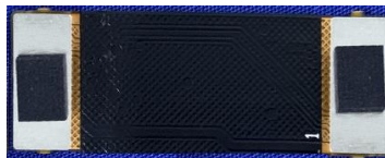
340-31973-000 ASSY, FPC, DISPLAY AND SHUTTER, CPPM1
