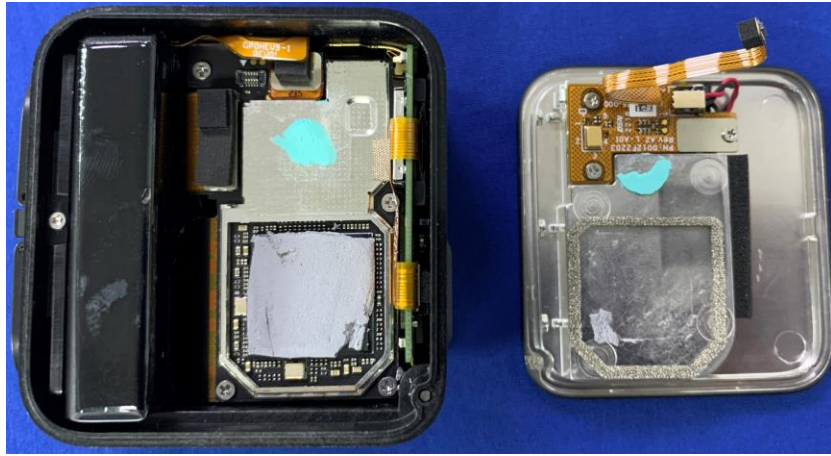
Rear cover, Mic, Speaker removed, CPPM1
