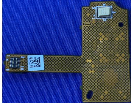
340-31974-000 ASSY, FPC, FRONT MIC AND MODE, CPPM1
