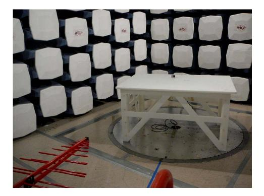
15.4 Radiated Emission below 1 GHz Rear View
