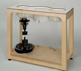
The DASY device holder has been made out of low-loss POM material having the following dielectric parameters: relative permittivity "=3 and loss tangent \_=0.02. The amount of dielectric material has been reduced in the closest vicinity of the device, since measurements have suggested that the influence of the clamp on the test results could thus be lowered.
