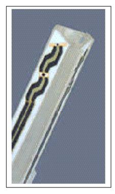
Inside view of ET3DV6 E-field Probe
