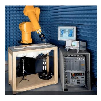
The system is based on a high precision robot (working range greater than 0.9m), which positions the probes with a positional repeatability of better than  $\pm 0.02mm$ . Special E- and H-field probes have been developed for measurements close to material discontinuity, the sensors of which are directly loaded with a Schottky diode and connected via highly resistive lines to the data acquisition unit.
