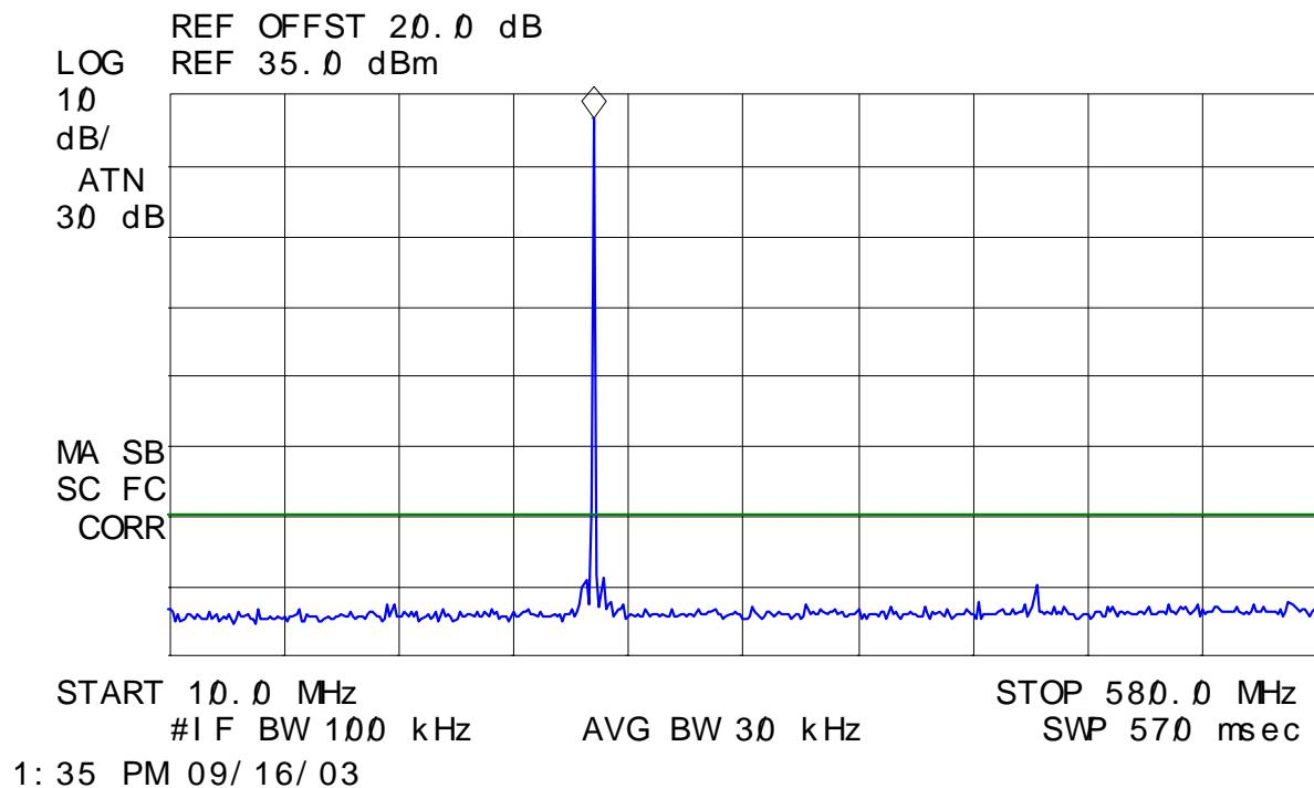
**Plot # 12: Transmitter RF Conducted Emissions at the Antenna Port**
