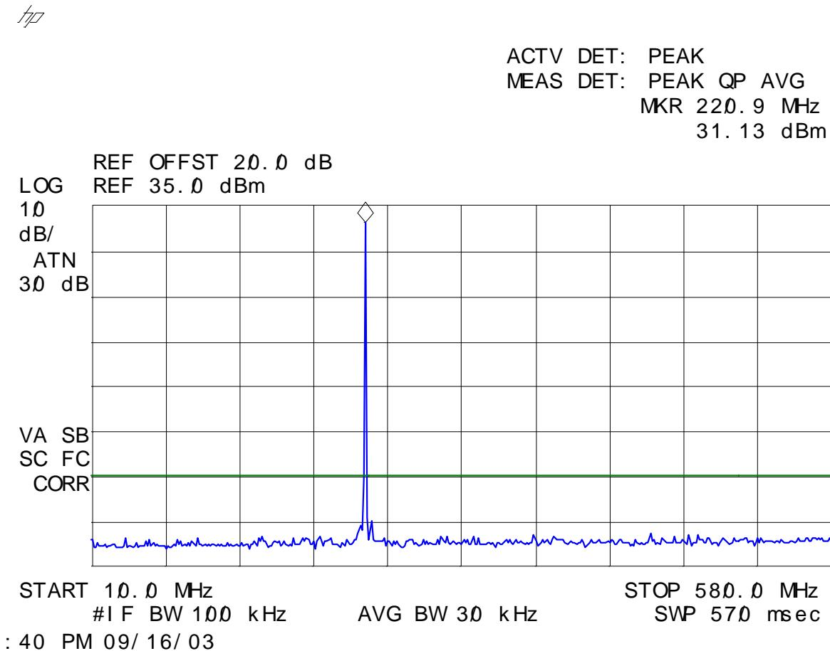
**Plot # 14: Transmitter RF Conducted Emissions at the Antenna Port**
