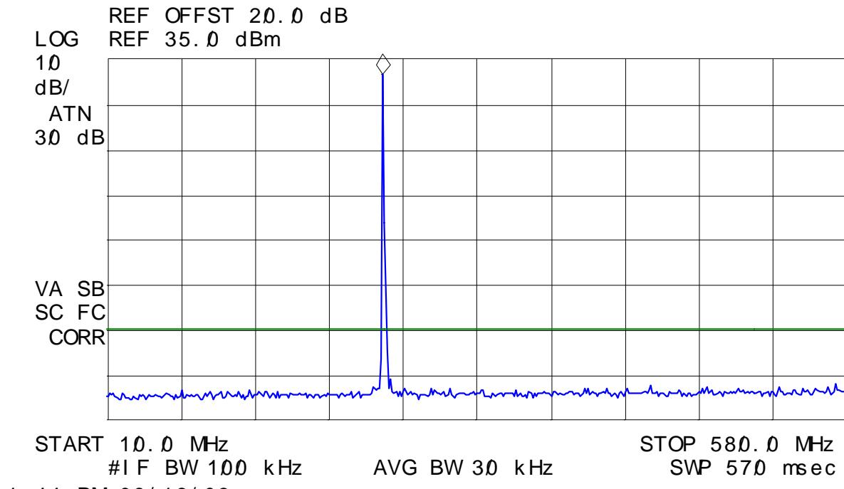
**Plot # 16: Transmitter RF Conducted Emissions at the Antenna Port**
