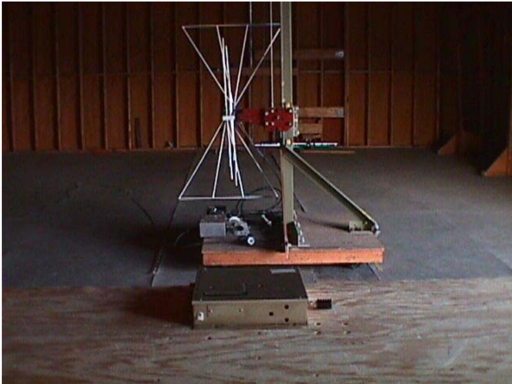
**ANNEX 1 - PHOTOGRAPHS OF TEST SETUP FOR RADIATED EMISSIONS**
