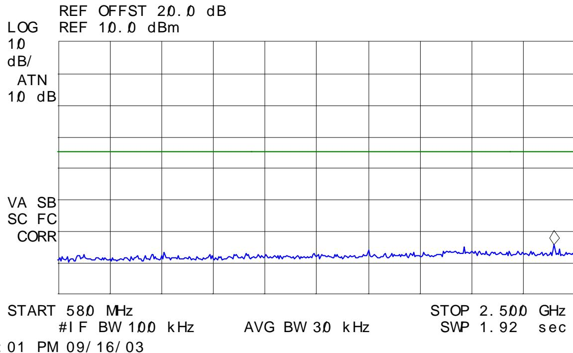
**Plot # 13: Transmitter RF Conducted Emissions at the Antenna Port**
