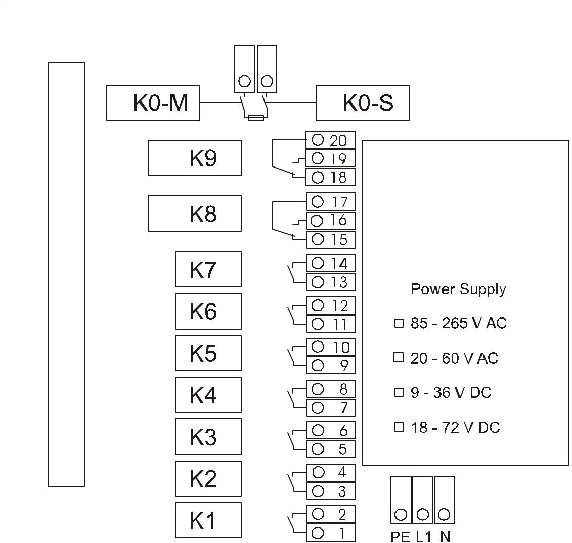
C-3 Connection Plan for Receiver with 12/17 Command Relays
