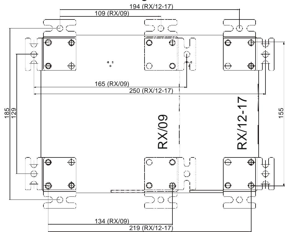
C-2 Connection Plan for Receiver with 9 Command Relays
