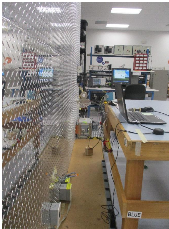
Figure 2: § 15.207(a) Conducted Emissions Limits, Test Setup Rear View
