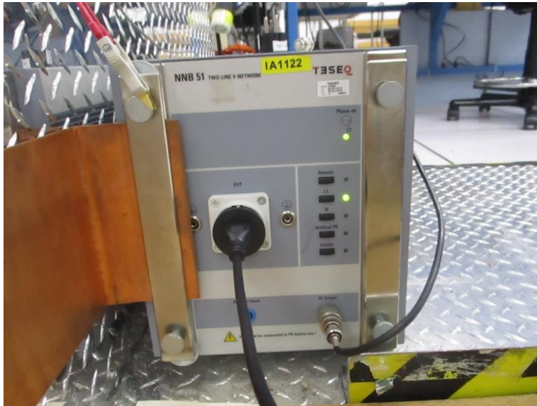
Figure 3: § 15.207(a) Conducted Emissions Limits, Test Setup LISN View
