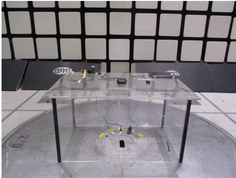
Figure 4: § 15.209 Radiated Spurious Emissions, 30-1000 MHz, Test Setup Front View
