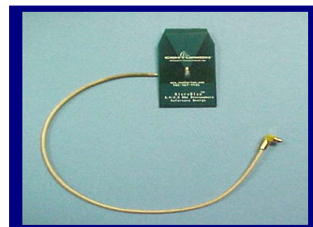
MicroBlue 2.4 shown here with standard 8 inches of RG-178 coax and right angle MMCX connector
