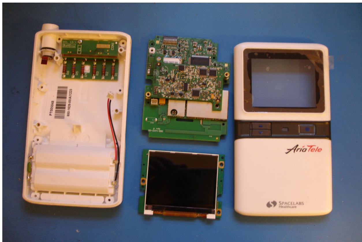
Figure 5: Transmitter 96281-C with Display PCBA removed SPO2 board fitted
