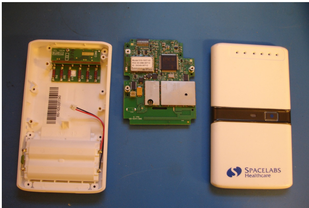
Figure 9: 96281-A components – this option uses the Main PCBA only
