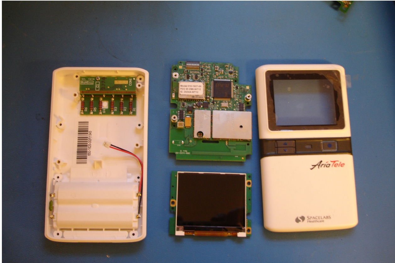
Figure 8: 96281-B components – Main PCBA and Display PCBA
