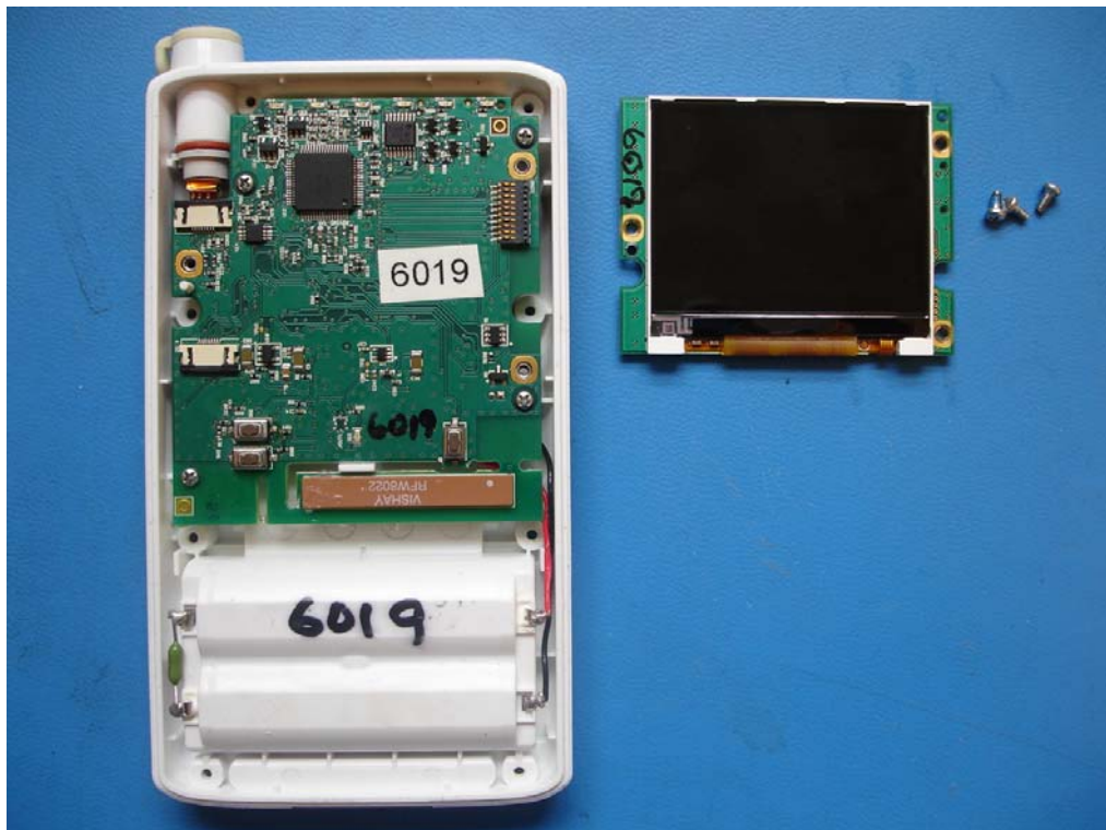
Figure 5: Transmitter 96281-C with Display PCBA removed
