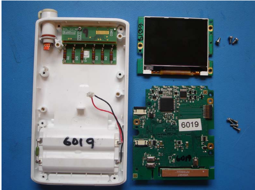
Figure 6: Transmitter 96281-C with Main PCBA and Display PCBA removed
