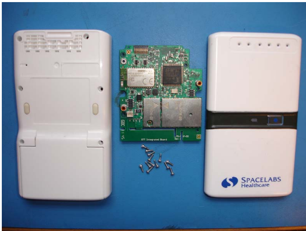
Figure 9: 96281-A components – this option uses the Main PCBA only
