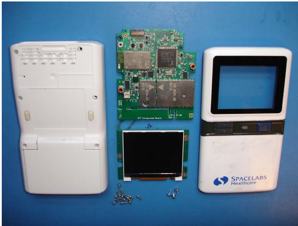
Figure 8: 96281-B components – Main PCBA and Display PCBA
