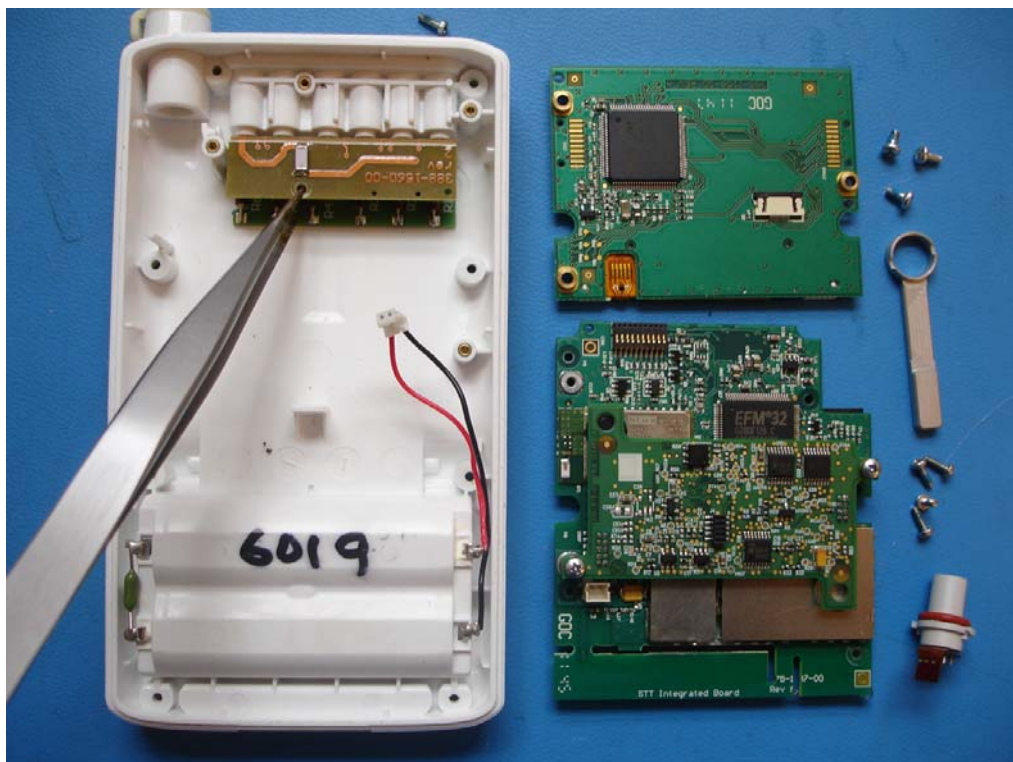
Figure 7: Transmitter 96281-C showing reverse side of PCBAs
