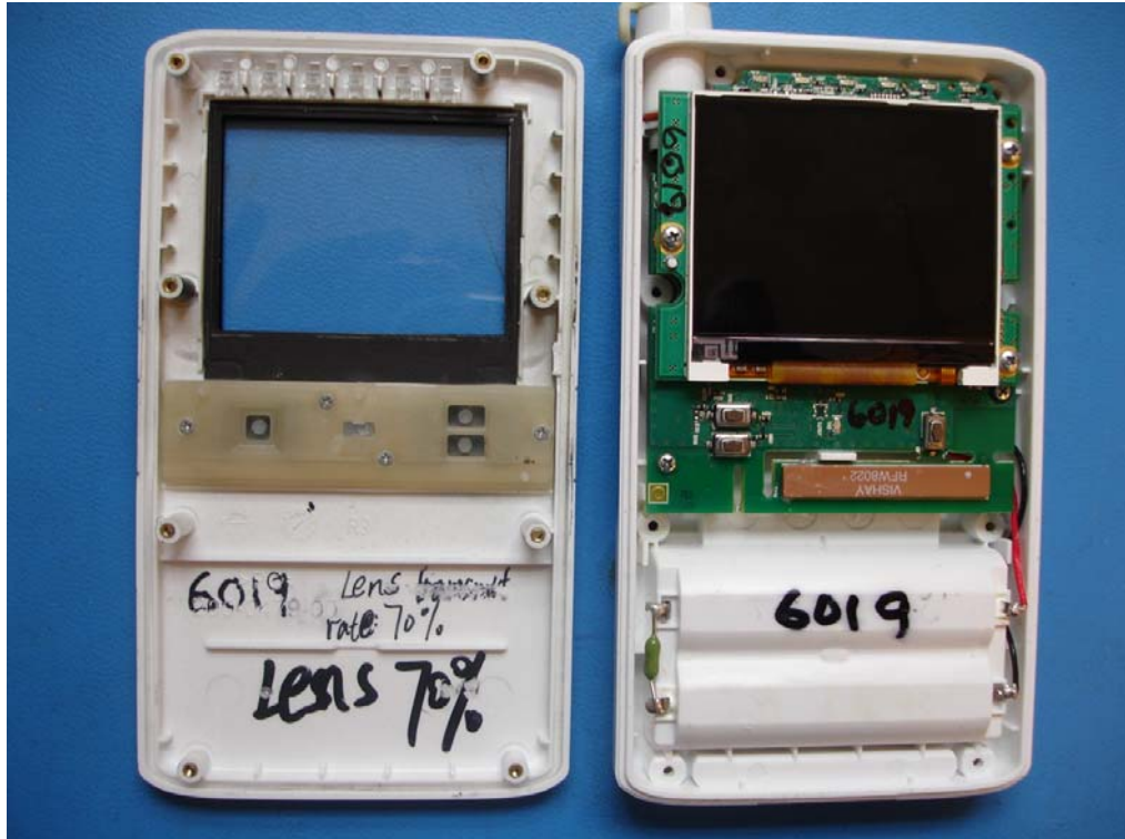
Figure 4: Transmitter 96281-C assembly with front cover removed
