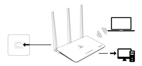
**Scenario 3:** Data service from Ethernet cord and VOLTE voice using a SIM card
