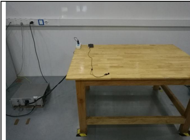
Conducted Emissions Test Setup Front View
