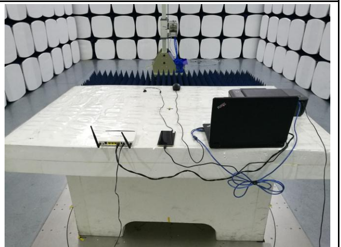
Radiated Emissions Test Setup Above 1GHz
