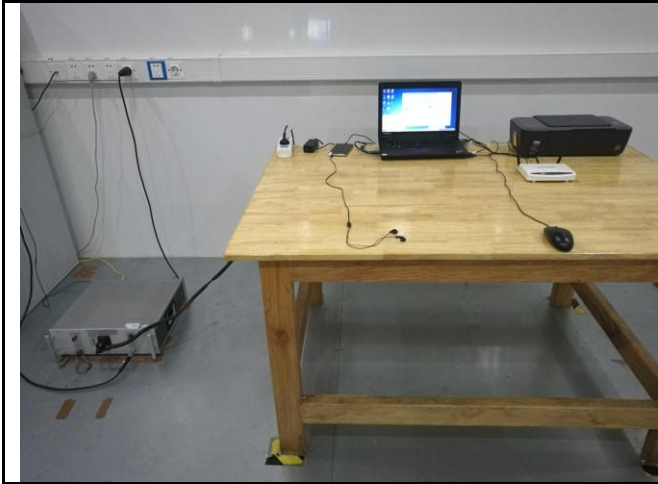
Conducted Emissions Test Setup – Front View
