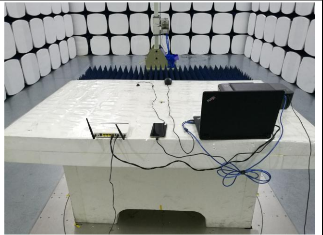
Radiated Emissions Test Setup Above 1GHz
