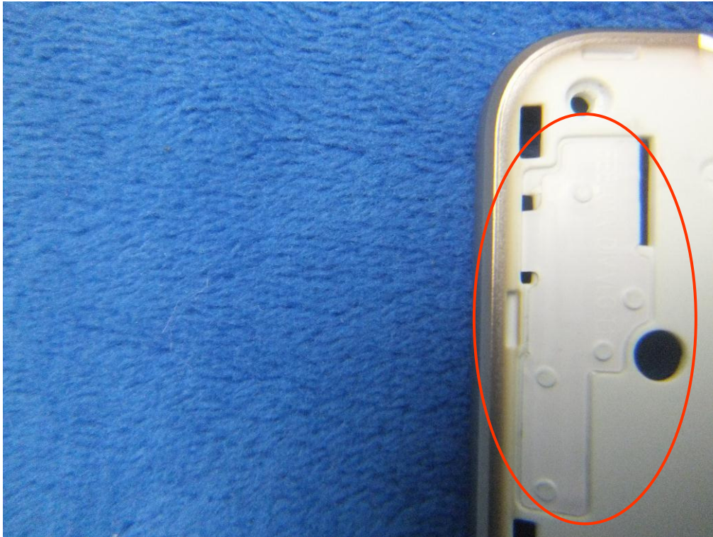
LTE - Antenna View
