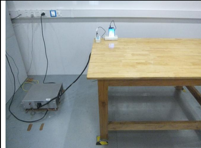
Conducted Emissions Test Setup Front View
