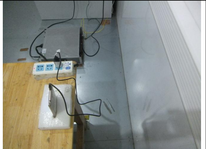
Conducted Emissions Test Setup Side View
