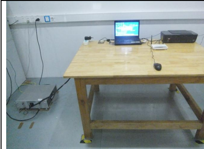
Conducted Emissions Test Setup – Front View
