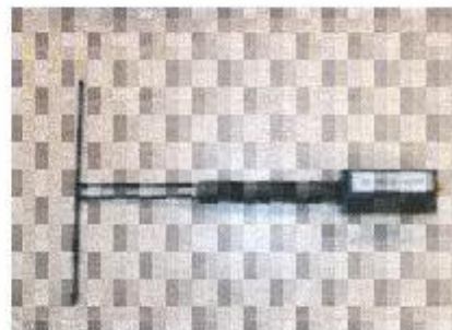
Figure 1 – Satimo COMOSAR Validation Dipole
