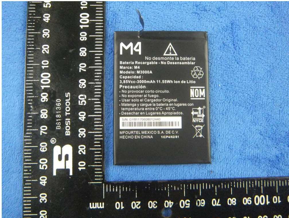
Battery - Front View
