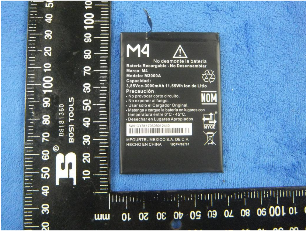
Battery - Front View
