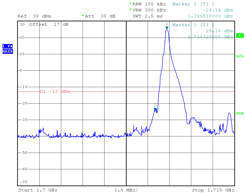
Lower Band Edge Plot for 16QAM -RB Size 1, RB Offset 0
