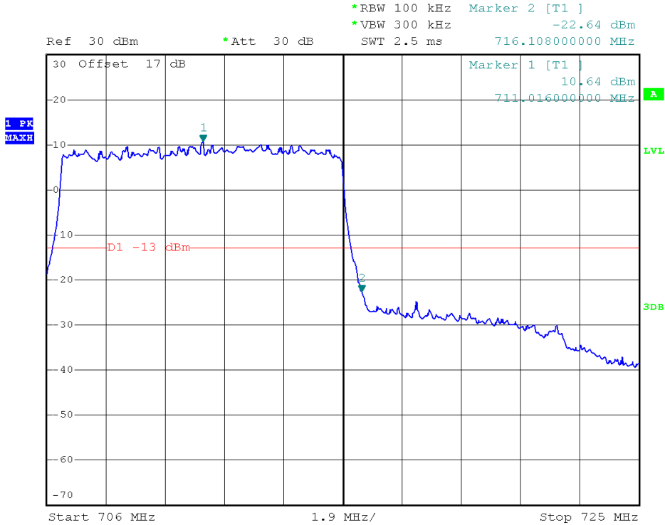
Higher Band Edge Plot for QPSK -RB Size 100, RB Offset 0
