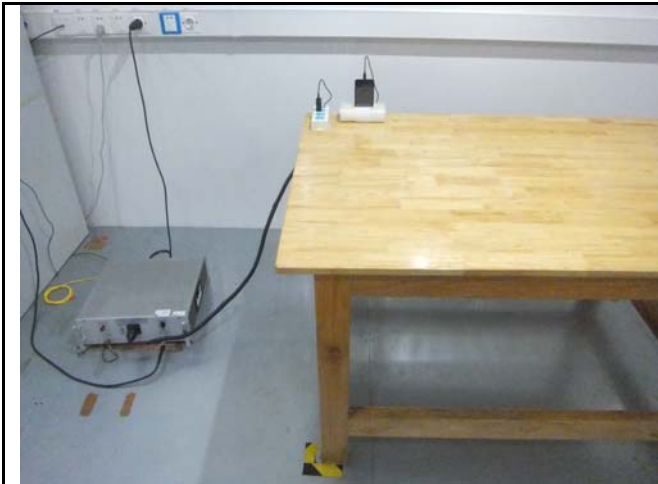
Conducted Emissions Test Setup Front View
