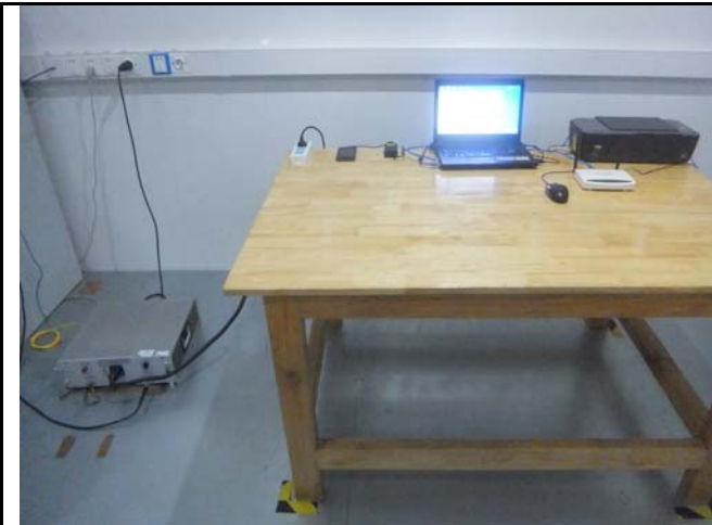
Conducted Emissions Test Setup – Front View
