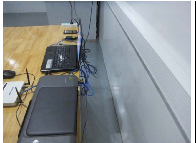
Conducted Emissions Test Setup – Side View
