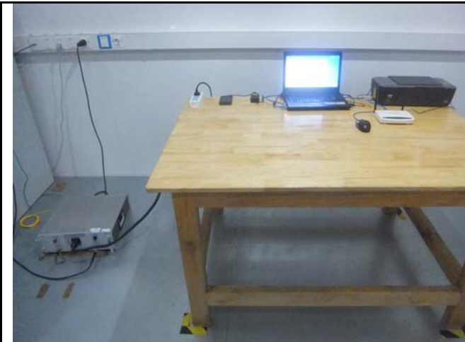
Conducted Emissions Test Setup – Front View
