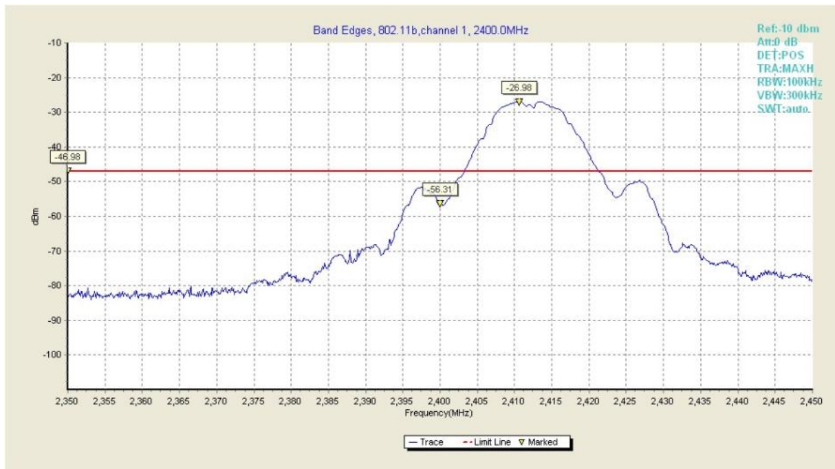
Fig25. Frequency Band Edges of 802.11b in channel 1,2400MHz
