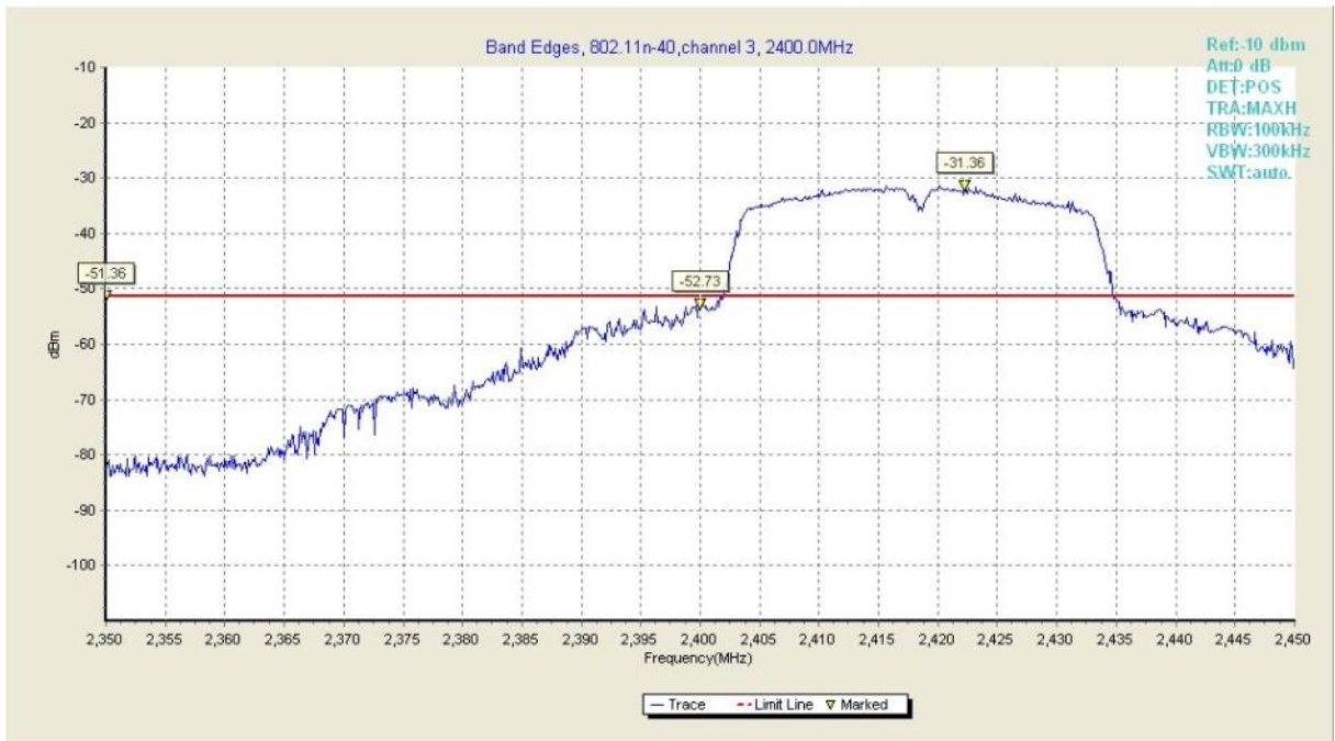
Fig31. Frequency Band Edges of 802.11n-40 in channel 1,2400MHz
