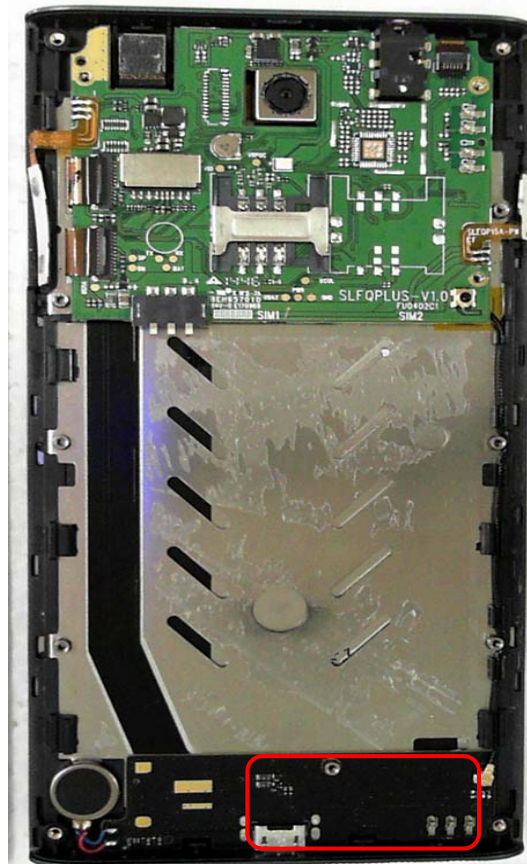
GSM/DCS/UMTS Antenna View
