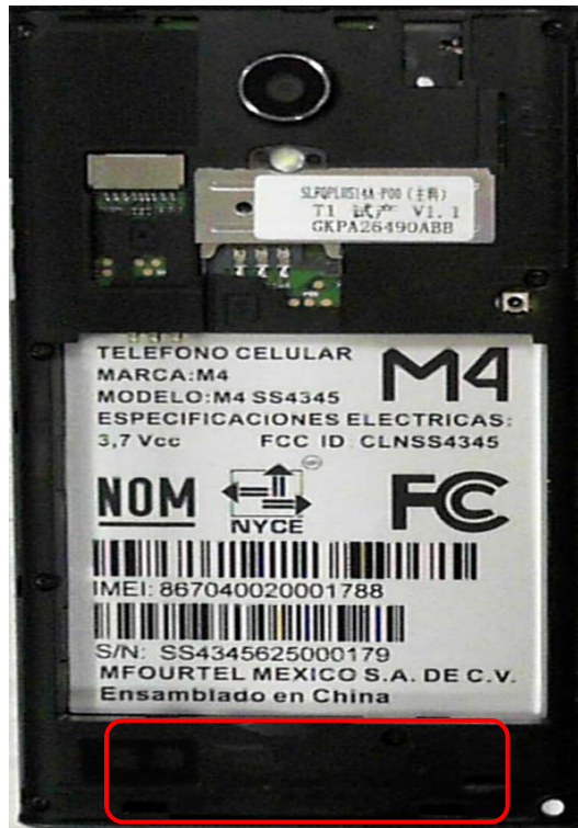
GSM/DCS/UMTS Antenna View
