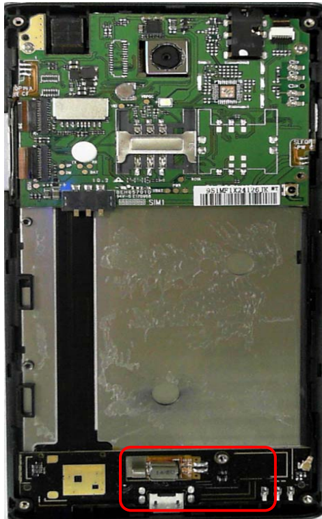
GSM/DCS/UMTS Antenna View
