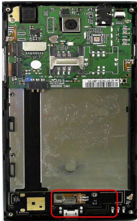
GSM/DCS/UMTS Antenna View
