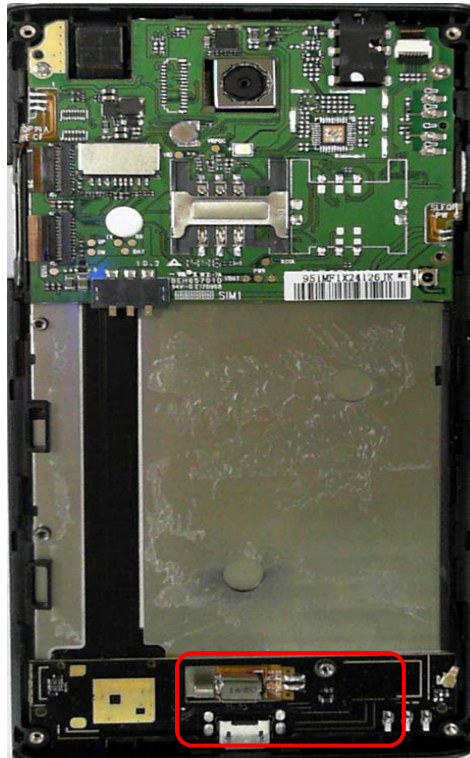
GSM/DCS/UMTS Antenna View
