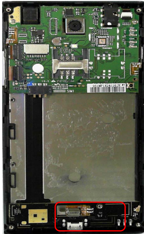
GSM/DCS/UMTS Antenna View
