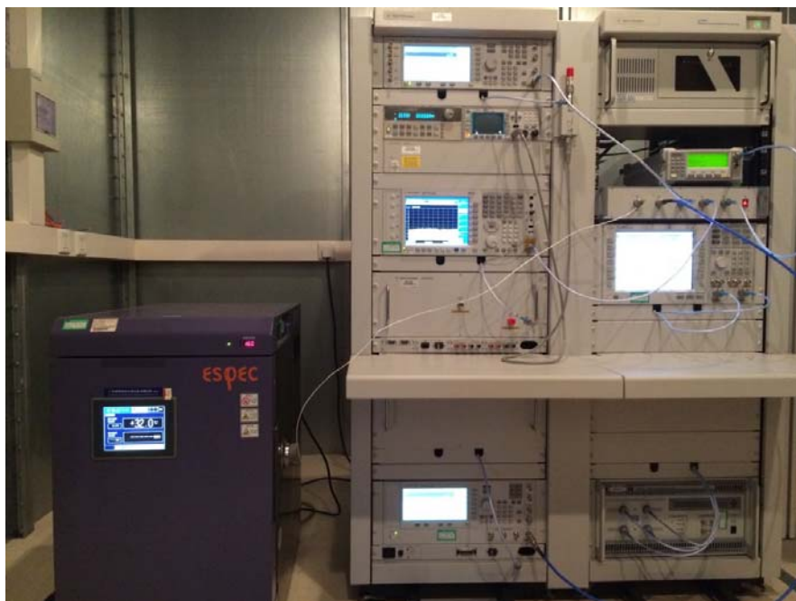
RF setup in extreme condition
