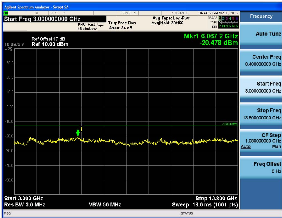
Fig.44 GSM1900 on Channel 661 3GHz~19.1GHz
