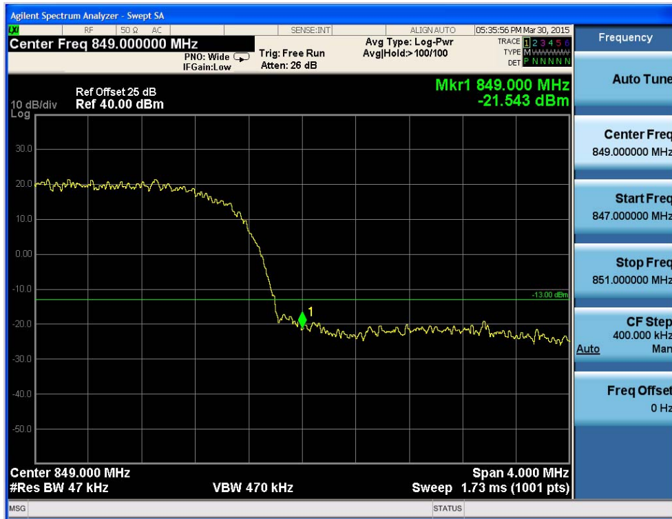
Fig.30 WCDMA Band V-CH4232 Band Edge Compliance
