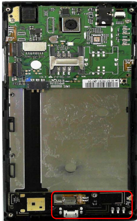
GSM/DCS/UMTS Antenna View
