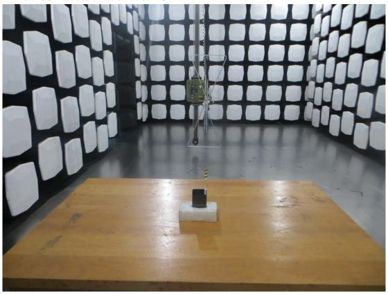
2. Part 15C Radiated emission above 1GHz
