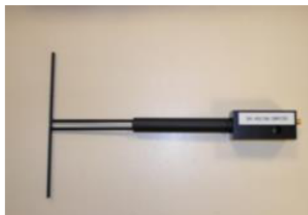
Figure 1 – Satimo COMOSAR Validation Dipole
