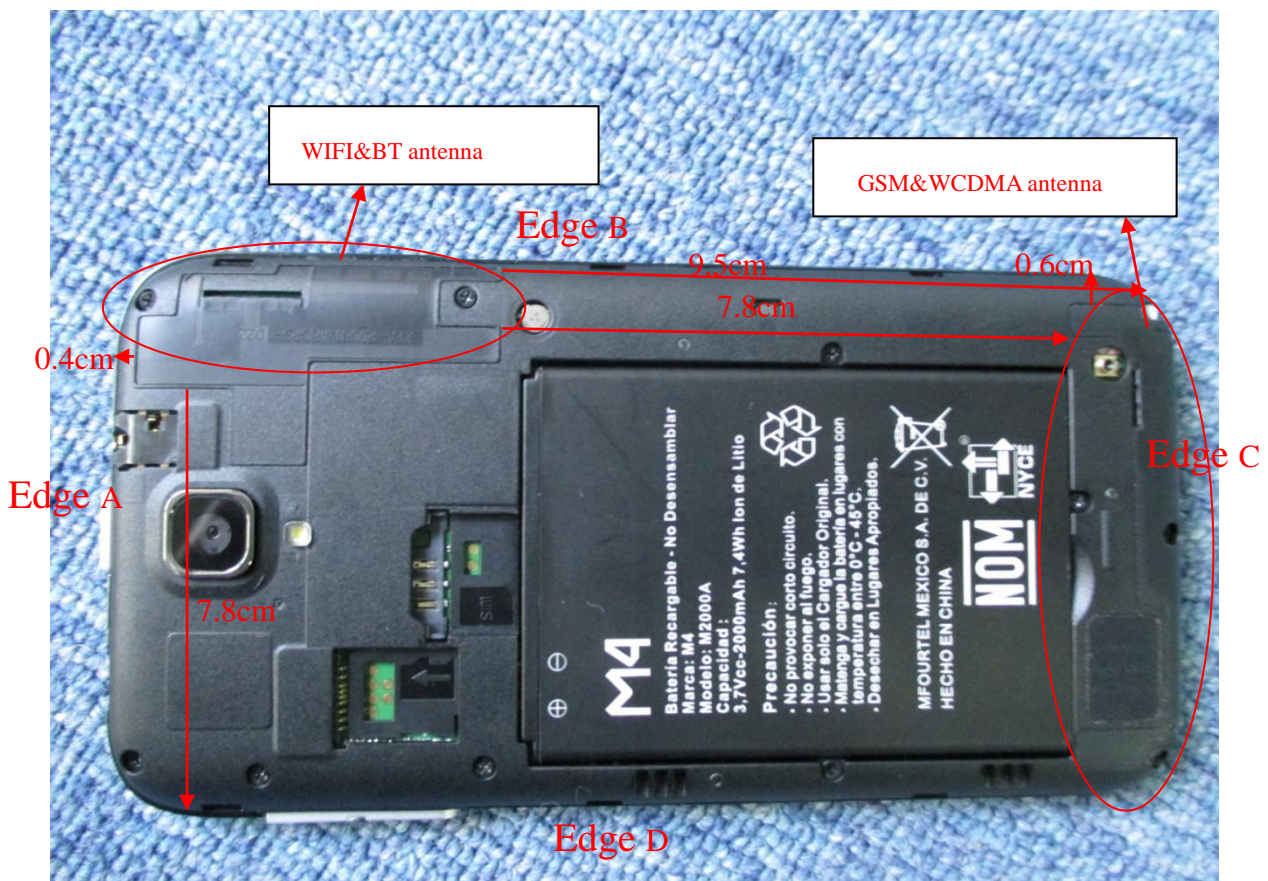
Fig. 3 Position of the antennas
