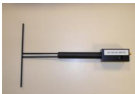
Figure 1 – Satimo COMOSAR Validation Dipole
