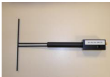
Figure 1 – Satimo COMOSAR Validation Dipole
