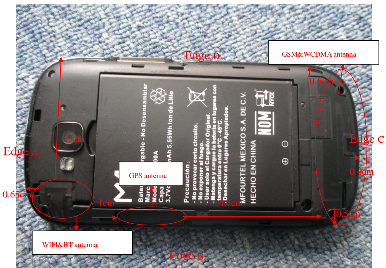
Fig. 3 Position of the antennas
