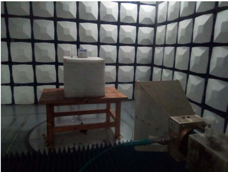
Radiated Emission View---Above 1GHz
