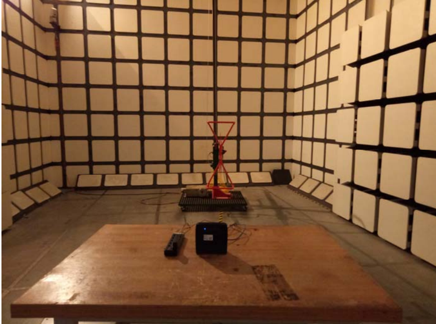
Radiated Emissions View (Below 1 GHz)
