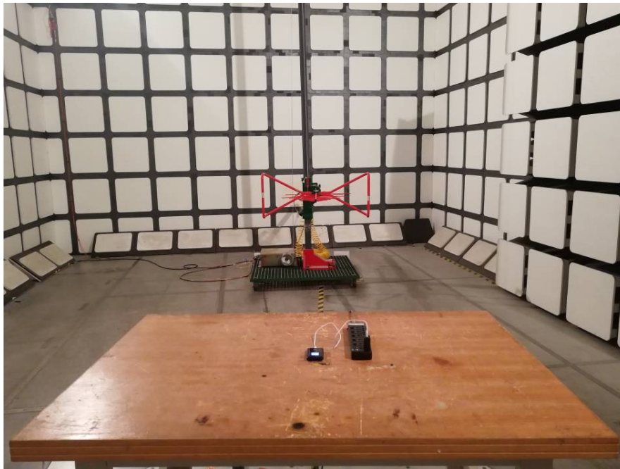
Radiated Emissions View (Below 1 GHz)
