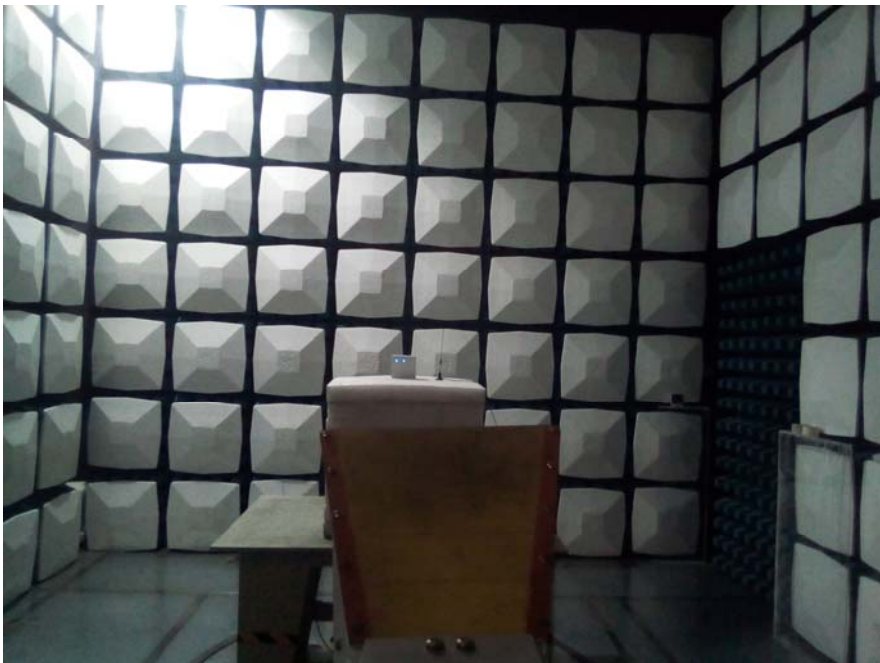
Radiated Emission View---Above 1GHz
