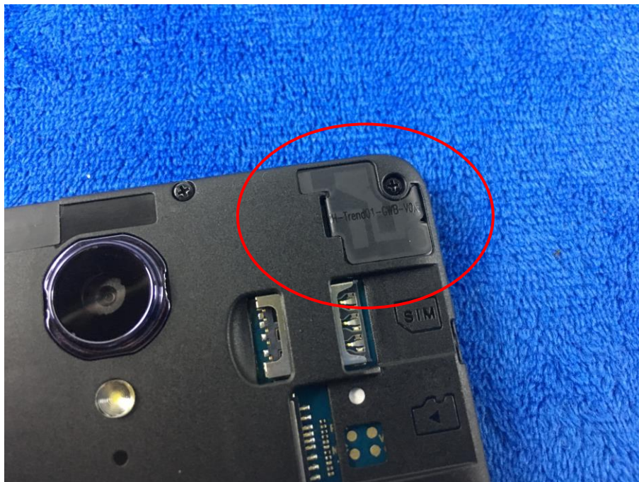
WIFI/BT/BLE/GPS - Antenna View
