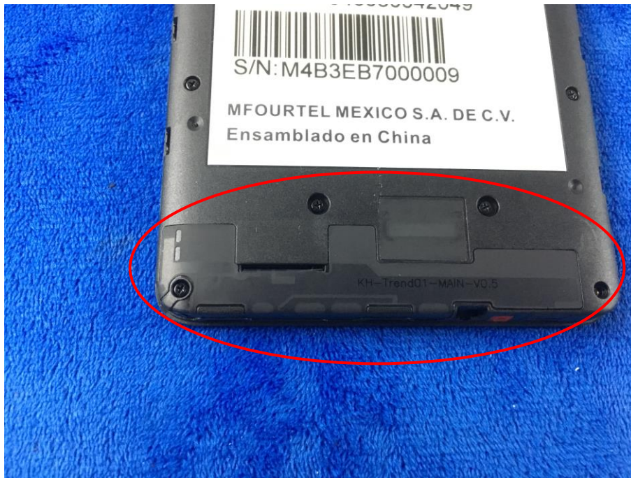
GSM/PCS/UMTS-FDD/LTE Antenna View
