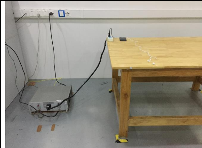
Conducted Emissions Test Setup Front View
